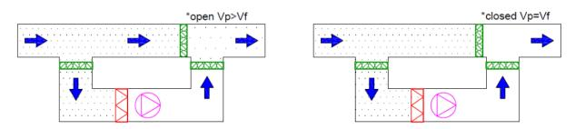
**Figure 2**. The idea of a cleaning device in the by-pass duct, based on [3a] \* – additional damper Vp – installation air flow, Vf – filter air flow
