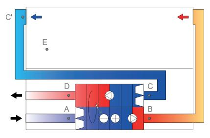
Figure 1. Locations of air cleaning devices (A, B, C, C', D, E).
